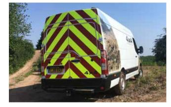
Master Red EDITION 4x4 is available in van and chassis cab derivatives at both 3.5 and 4.5 tonne GVW. They offer optimum traction in the most challenging areas but are switchable to 4x2 which reduces fuel consumption when on the open road.
